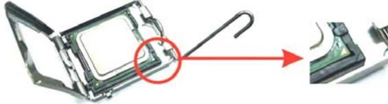
**Step 3:** Hold the CPU down firmly, and then close the lever to complete the installation.
