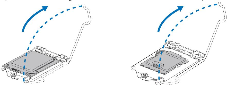
Step 3: Remove the Pin Cap.
