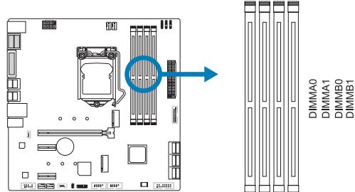
Step 1: Unlock a DIMM slot by pressing the retaining clips outward. Align a DIMM on the slot such that the notch on the DIMM matches the break on the slot.
