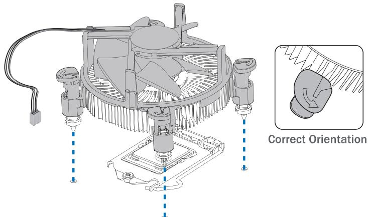
Step 2: Press down two fasteners at one time in a diagonal sequence to secure the CPU fan assembly in place. As each fastener locks into position a click should be heard.
