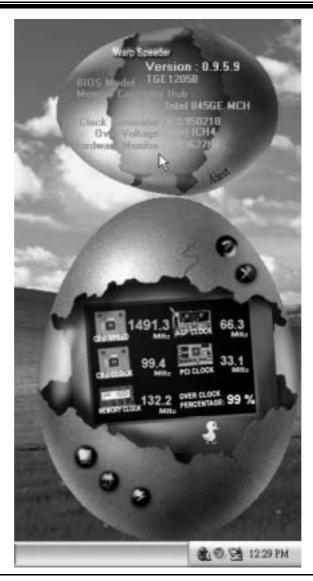
Note: Because the overclock, overvdtage, and hardware monitor features are controlled by several separate chipset, [WarpSpeeder ] divide these features to separate panels. If one chipset is not on board, the correlative button in Main panel will be disabled, but will not interfere other panels' functions. This property can make [WarpSpeeder ] utility more robust.
