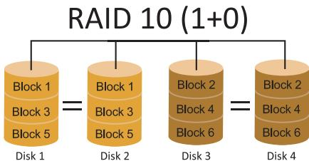
RAID 10 combines the advantages (and disadvantages) of RAID 0 and RAID 1 in one single system. It provides security by mirroring all data on a secondary set of disks (disk 3 and 4 in the drawing below) while using striping across each set of disks to speed up data transfers.
