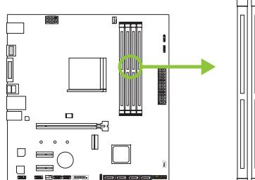
**Step 1:** Unlock a DIMM slot by pressing the retaining clips outward. Align a DIMM on the slot such that the notch on the DIMM matches the break on the slot.
