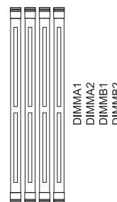
**Step 2:** Insert the DIMM vertically and firmly into the slot until the retaining clips snap back in place and the DIMM is properly seated.
