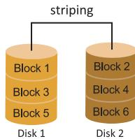
In a RAID 0 system data are split up in blocks that get written across all the drives in the array. By using multiple disks (at least 2) at the same time, this offers superior I/O performance. This performance can be enhanced further by using multiple controllers, ideally one controller per disk.
