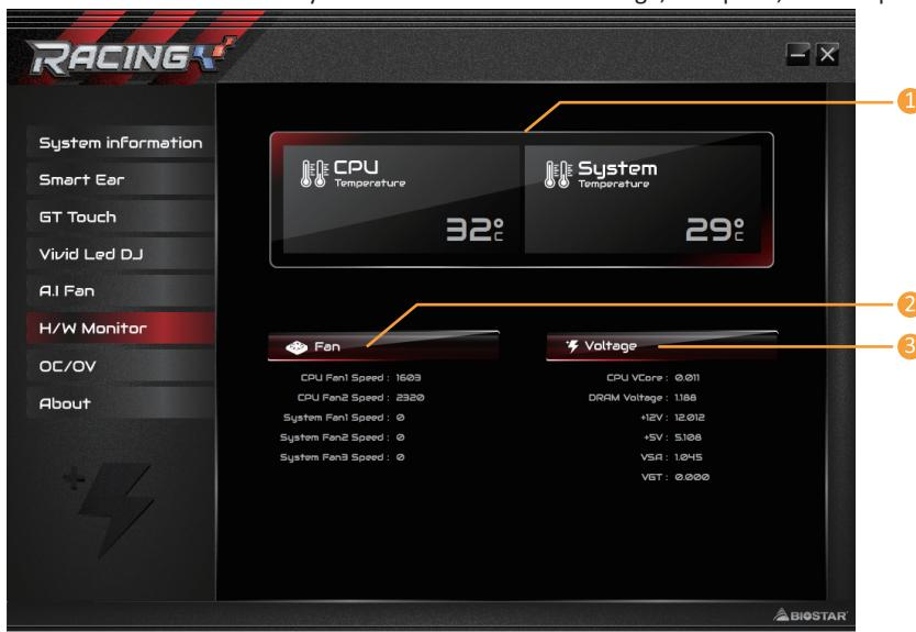
1. **CPU Temperature/System Temperature:** Shows the current CPU and system temperature.
