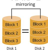
Data are stored twice by writing them to both the data disk (or set of data disks) and a mirror disk (or set of disks). If a disk fails, the controller uses either the data drive or the mirror drive for data recovery and continues operation. You need at least 2 disks for a RAID 1 array.
