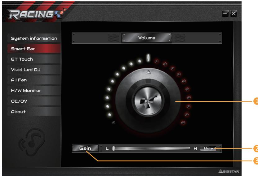
**1. Volume Control Knob:** The volume can be finely adjusted by turning the knob either clockwise or anti-clockwise to increase or decrease system volume accordingly.
