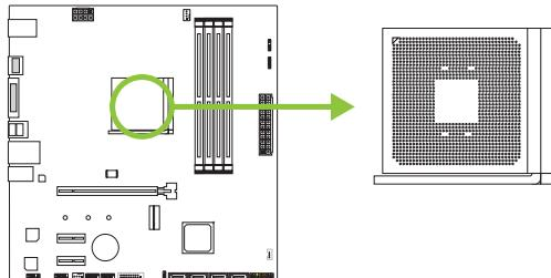
Step 2: Pull the socket locking out from the socket and then raise the lever up to a 90-degree angel.
