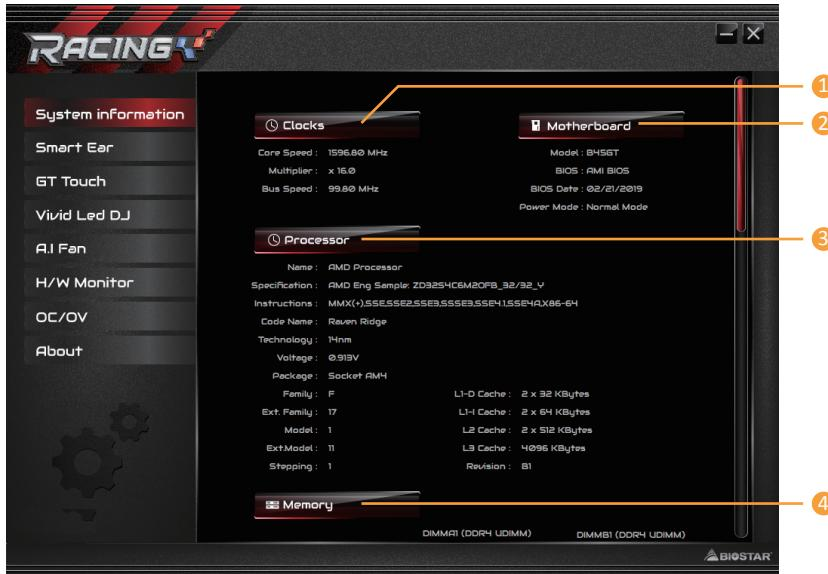
**1. Clocks:** Shows core speed, multiplier and bus speed.
