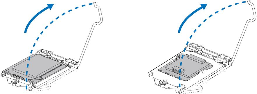
Step 3: Remove the Pin Cap.
