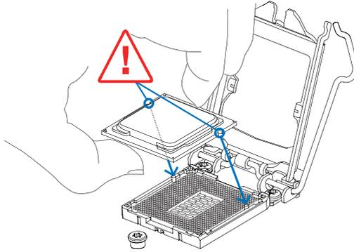
Step 5: Hold the CPU down firmly, and then lower the lever to locked position to complete the installation.
