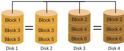
RAID 10 combines the advantages (and disadvantages) of RAID 0 and RAID 1 in one single system. It provides security by mirroring all data on a secondary set of disks (disk 3 and 4 in the drawing below) while using striping across each set of disks to speed up data transfers.
