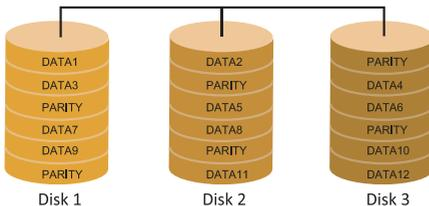
A RAID 5 array can withstand a single disk failure without losing data or access to data. Although RAID 5 can be achieved in software, a hardware controller is recommended. Often extra cache memory is used on these controllers to improve the write performance.
