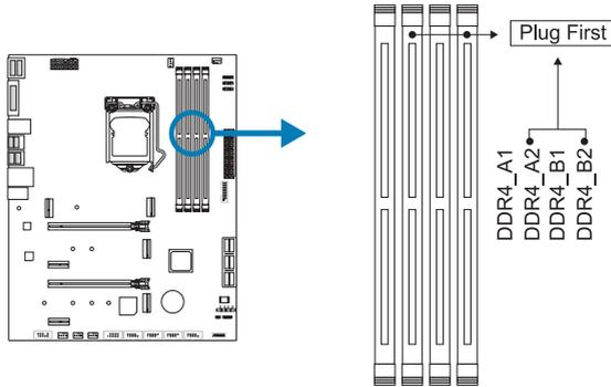
Step 1: Unlock a DIMM slot by pressing the retaining clips outward. Align a DIMM on the slot such that the notch on the DIMM matches the break on the slot.
