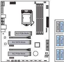
1x M.2 SATA SSD Slot + 2x M.2 PCIe SSD Slot
