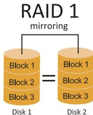
Data are stored twice by writing them to both the data disk (or set of data disks) and a mirror disk (or set of disks) . If a disk fails, the controller uses either the data drive or the mirror drive for data recovery and continues operation. You need at least 2 disks for a RAID 1 array.
