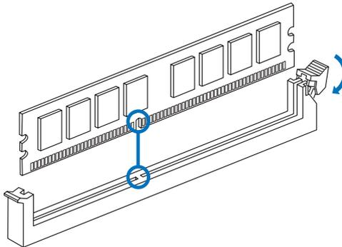
Step 2: Insert the DIMM vertically and firmly into the slot until the retaining clips snap back in place and the DIMM is properly seated.
